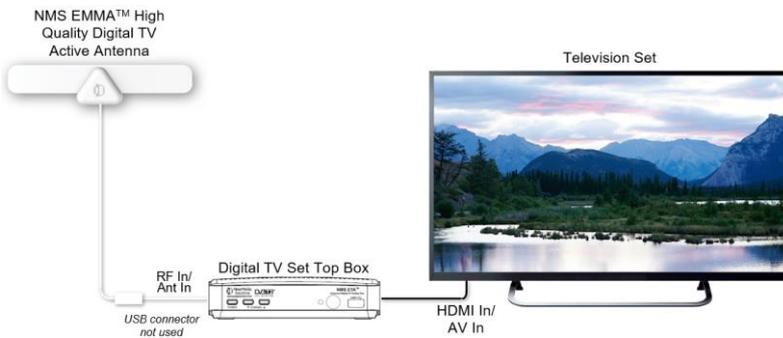
1. Connect the antenna's IEC connector to the RF In/Ant In port on your set-top Box.
